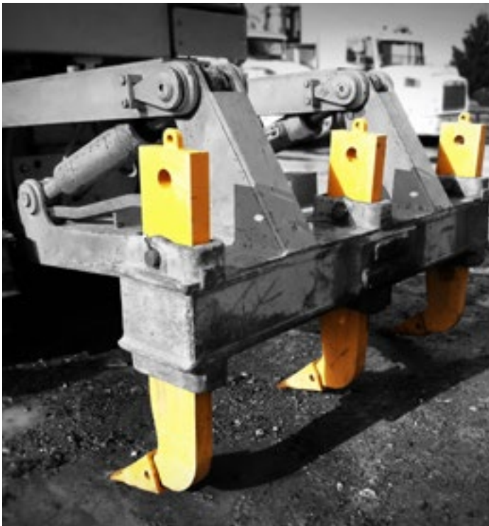
▲ Custom-made 75mm Hardox CAT D7 Ripper Shanks
